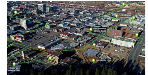
Figure 6 - Map of City of Prince George Downtown Renewable Energy System, indicating most of the distribution piping network and connected buildings.
