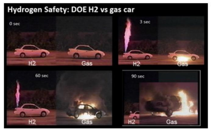
Testing conducted by the <u>U.S. Department of Energy</u> studying the burning characteristics of a vehicle with a hydrogen fuel tank (left) and a gasoline fuel tank (right).
